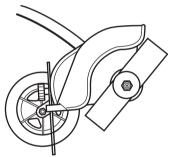
Check that the guard is undamaged and not cracked. Replace the guard if it has been exposed to impact or is cracked.
