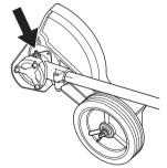
The grease in the bevel gear does not normally need to be changed except if repairs are carried out.
