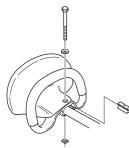
5 Now make a final adjustment to give yourself a comfortable working position. Tighten the screw. CAUTION! The loop handle and hand guard must not be fitted behind the arrow marked on the shaft.
