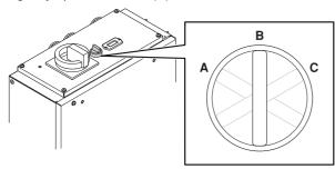
To activate the remote control mode, turn the knob to the left (A).
