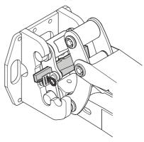
Connect the hydraulic hoses and any hoses for hammer lubrication (when fitting the hammer). Viewed from behind, the pressure connection of the tool should be connected on the left side (B port) and the return hose on the right side (A port).
