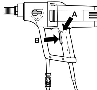
The power switch lock remains depressed as long as the power switch is depressed. When the grip on the handle is released both the power switch and power switch lock are reset. This movement is controlled by two independent return springs. This position results in the machine stopping and the power switch being locked.
