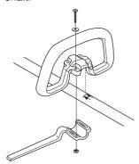
Finely adjust the J-handle to give a comfortable working stance. Tighten the screws.
