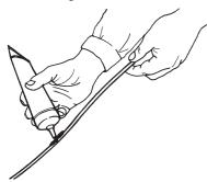
Slide the drive shaft back into the sleeve. Make sure the shaft engages correctly by turning it and pushing at the same time.
