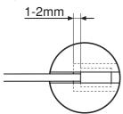
When the throttle cable is adjusted correctly, tighten the lock-nut (G).
