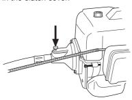
Remove the clip that holds the throttle wire against the drive shaft.
