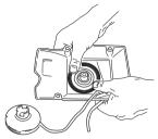
Lubricate the recoil spring with light oil. Fit the cassette with recoil spring in the starter. Fit the starter pulley and tension the recoil spring.
