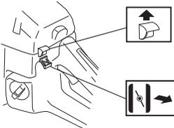
If the machine is fitted with a decompression valve (A): Press the valve to reduce the pressure in the cylinder and make starting easier. You should always use the decompression valve when starting the machine. Once
