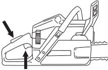
Note! Pull the front hand guard towards the front handle. The chain brake is now disengaged. Your saw is ready for use.
