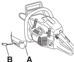
These reduce the flow of cooling air and prevent large amounts of snow from being sucked into the carburetor space.
