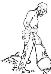
Keep the trunk between you and the chain saw as you move along the trunk.
