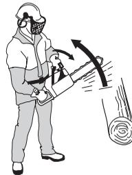
If the kickback is less violent or the kickback zone of the bar is closer to you the chain brake is designed to
