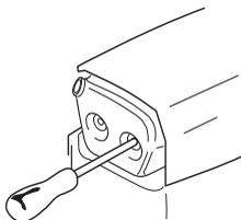
Some mufflers are equipped with a special spark arrester screen. If your machine has this type of muffler, you should clean the screen at least once a week. This is best done with a wire brush. A blocked screen will cause the engine to overheat and may lead to serious damage.
