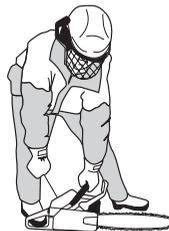
Push in the choke control as soon as the engine fires and make repeated starting attempts. Immediately press and release the throttle when the engine starts. That will disengage the throttle latch.
