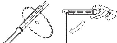
Check the cutting attachment for damage or cracks. A damaged cutting attachment should always be replaced.
