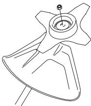
When fitting, tighten the nut in the opposite direction to the direction of rotation of the cutting attachment. To remove it, undo the nut in the same direction as the cutting attachment rotates. (CAUTION! The nut has a left-hand thread.) Tighten the nut using the socket spanner.
