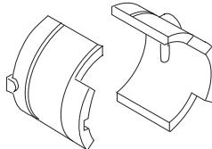
Regularly check the vibration damping units for cracks or deformation. Check that the vibration damping element is undamaged and securely attached.
