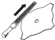
Keep the correct setting on the saw blade! Follow our instructions and use the recommended setting tool. An incorrectly set saw blade increases the risk of jamming and blade thrust, and damage to the saw blade.
