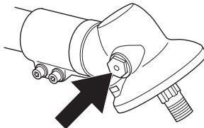
The grease in the bevel gear does not normally need to be changed except if repairs are carried out.
