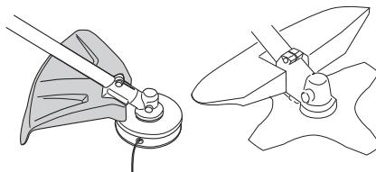
Check that the guard is undamaged and not cracked. Replace the guard if it has been exposed to impact or is cracked.
