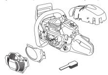
Clean the cooling system with a brush once a week, more often in demanding conditions. A dirty or blocked cooling system results in the machine overheating which causes damage to the piston and cylinder.
