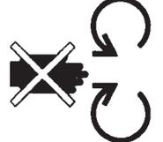
Rotary blades Keep hands and feet away from under the hood when the engine is running
