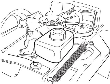
**Rider 18.** Fill if necessary with engine oil SAE 10W/40 (class SF-CC).
