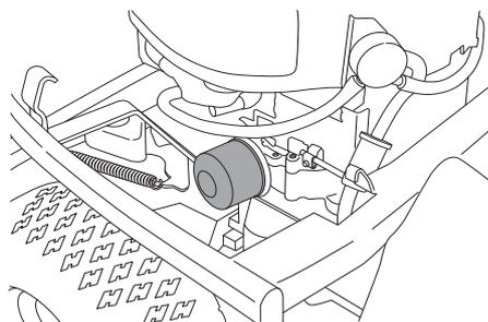
Lightly lubricate the rubber seal on the new oil filter using new oil. Fit the oil filter by turning clockwise. Turn by hand until the rubber seal is seated. Now tighten a further half turn.
