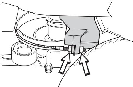
Hold the cable, for example using an adjustable wrench, so that it does not twist.
