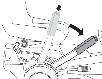
The lever can also be used to temporarily regulate the cutting height, e.g. for a small mound in the lawn.
