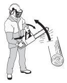
If the kickback is less violent or the kickback zone of the bar is closer to you the chain brake is designed to be activated manually by the movement of your left hand.
