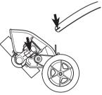
Position the angle gear so that its slot is aligned with the line on the supporting tube.
