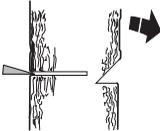
Finish the felling cut parallel with the directional cut line so that the distance between them is at least 1/10 of the trunk diameter. The uncut section of the trunk is called the felling hinge.
