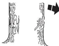
Next make the bottom cut so that it finishes exactly at the end of the top cut.
