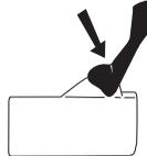
Move the front hand guard forwards and back to make sure it moves freely and that it is securely anchored to the clutch cover.
