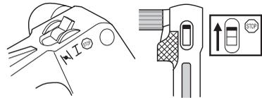
The engine is stopped by pushing the stop switch to the stop position.
