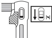
**Primer bulb:** Press the air purge repeatedly until fuel begins to fill the bulb. The bulb need not be completely filled.
