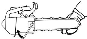
When fitting a new chain, the chain tension has to be checked frequently until the chain is run-in. Check the chain tension regularly. A correctly tensioned chain ensures good cutting performance and long life.
