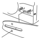
Tension the chain by turning the chain tensioning screw clockwise using the combination spanner. The chain should be tensioned until it does not sag from the underside of the bar. See instructions under the heading Tensioning the chain.
