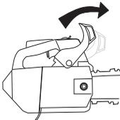
**Ignition; choke:** Slide the control to its rear position.
