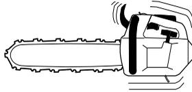
Make sure the vibration damping units are securely attached to the engine unit and handle unit.
