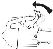
Unscrew the bar nut and remove the clutch cover (chain brake). Take off the transportation guard.
