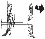
Set the spike bumper (if one is fitted) just behind the felling hinge. Use full throttle and advance the chain/bar slowly into the tree. Make sure the tree-top does not start to move in the opposite direction to your intended felling direction.
