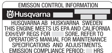
The Emissions Compliance Period referred to on the Emission Compliance label indicates the number of operating hours for which the engine has been shown to meet Federal and Californian emissions requirements.
