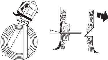
Use full throttle and bring the bar and chain slowly into the tree. Make sure the tree does not start to move in the opposite direction to your intended felling direction. Drive a wedge or breaking bar into the cut as soon as it is deep enough.
