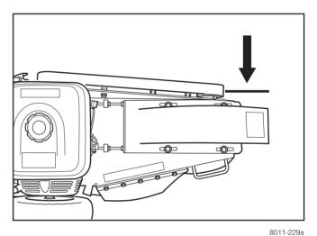
Check clutch and pulley alignment using inside face
