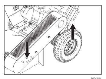
The lifting handles can also be used to secure the machine for transport.
