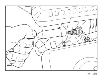
Remove the spark plug cable.
