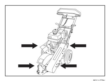
Lift the machine with the side handles.
