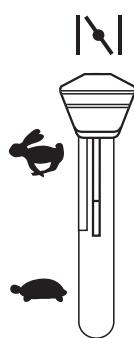
(GB) Cold motor: Push the gas control up to end positon choke (↖).
