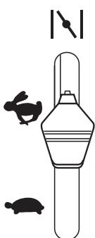
GB Warm motor: Push the gas control half-way to full gas position "F".
