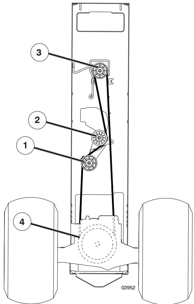
GB Assemble in the reverse order to dismantling. Check that the belt lies inside all the belt guides. Use original belts only when replacing!
