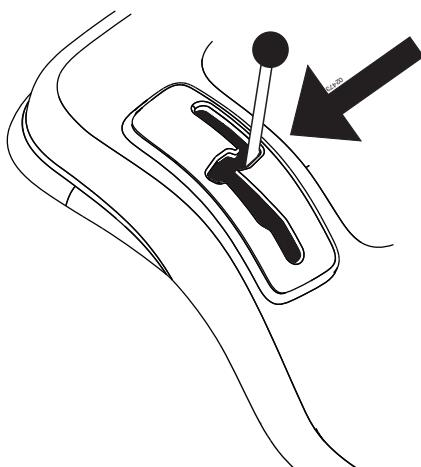
(GB) Press down the clutch/brake pedal completely and hold down. Set the gear lever in neutral "N".
