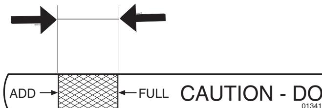
GB The oil level should lie between the two markings on the oil stick. If more oil is needed add SAE 30 oil to the "FULL" marking. SAE 5W-30 oil should be used during the winter (below freezing point).
