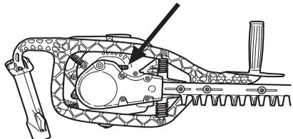
**CAUTION!** The gear housing must not be filled completely with grease. The grease expands as the machine heats up during operation. If the gear housing was completely filled with grease it could damage the seals and lead to leakage of grease.
