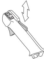
Check that the throttle control and throttle lockout move freely and that the return springs work properly.
