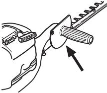
Check that the hand guard is fitted correctly.
