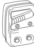
In countries that have a warm and dry climate there is a significant risk of fire. We therefore fit certain mufflers with a spark arrester mesh. Check whether the muffler on your machine is fitted with this kind of mesh.
