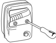
If the muffler on your machine is fitted with a spark arrester mesh this must be cleaned regularly. A blocked mesh will cause the engine to overheat and may lead to serious damage.
