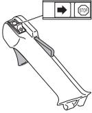
Start the engine and make sure the engine stops when you move the stop switch to the stop setting.
