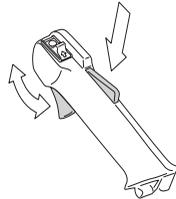
See instructions under the heading Start. Start the hedge trimmer and apply full throttle. Release the throttle trigger and check that the blades stop and remain stationary. If the blades move when the throttle trigger is in the idle position then the carburettor idle setting must be adjusted. See instructions under the heading Maintenance.
