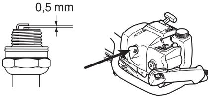
**CAUTION!** Always use the recommended spark plug type! Use of the wrong spark plug can damage the piston/cylinder. Check that the spark plug is fitted with a suppressor.
