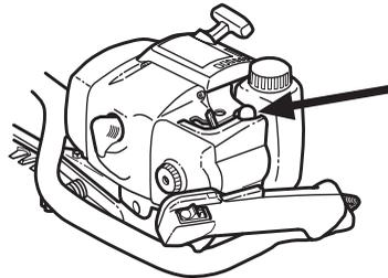
**Choke:** Set the choke control in the choke position.
