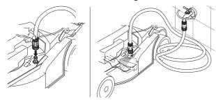
Start the engine and let the blade rotate for a while. The water is thrown out and cleaning the cutting cover.
