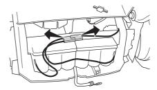
Connect the battery charger and charge the battery for max. 24 hours.
