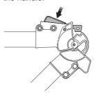
· Adjust the height of the top part of the handlebar.
