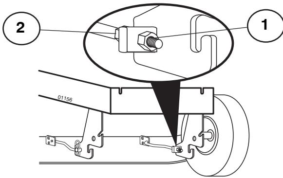
**GB** To achieve best cutting results the cutting unit's front edge (B) should be about 10 mm (0.375") lower than the back edge (A). Adjust in the following way to raise the back edge:
