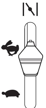
GB Warm motor: Push the gas control half-way to full gas position "↑".
