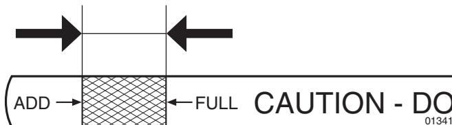
**GB** The oil level should lie between the two markings on the oil stick. If more oil is needed add SAE 30 oil to the "FULL" marking. SAE 5W-30 oil should be used during the winter (below freezing point).
