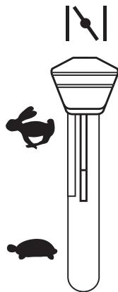
GB Cold motor: Push the gas control up to end positon choke (↑).
