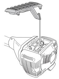
IMPORTANT! If the temperature rises above -5°C (23°F) or 0°C (32°F) respectively the machine MUST be restored to its normal set-up. Otherwise there is a risk of overheating, which can cause severe engine damage.
