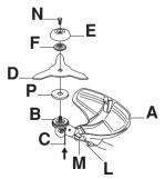
Screw the support cup (E) onto the output shaft threads (CAUTION! Left-hand thread). Tighten to a torque of 35-50 Nm (3.5-5.0 kpm). Use the socket spanner in the tool kit. Note that the locking pin (C)
