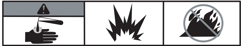
Battery acid is corrosive, explosive and flammable
