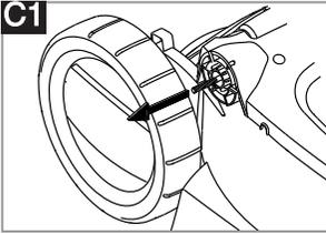
1. Pull the lower handle bolt until it locks into position as illustrated in **fig C1**.
