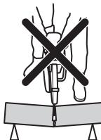
If the blade is pinched or stalled in the kickback zone, the reactive force will push the power cutter up and back towards the user in a rotating motion causing serious or even fatal injury.
