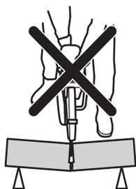
If the blade is pinched or stalled in the kickback zone, the reactive force will push the power cutter up and back towards the user in a rotating motion causing serious or even fatal injury.
