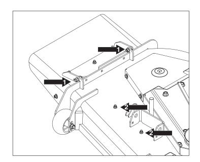
4. Bolt left hand corner mulch baffle to the **outside** of the deck baffle weldment as shown in the illustration.
