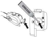
3 Fill with grease by putting the tube of grease as far into the hole as possible, and fill until grease starts to trickle out of the hole.
