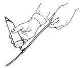
5 Slide the drive shaft back into the sleeve. Make sure the shaft engages correctly by turning it and pushing at the same time.
