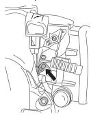
6 To adjust, turn the adjustment screw (B) clockwise and try point 5 again until the carburettor throttle cam bottoms at maximum throttle setting.
