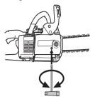
Use the combination spanner to tighten the bar nuts while lifting the tip of the bar at the same time. Check that you can pull the chain round freely by hand and that it does not sag from the underside of the bar.
