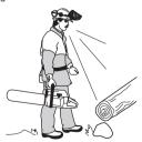
5 Take great care when cutting a tree that is under tension. A tree that is under tension may spring back to its normal position before or after being cut. If you position yourself incorrectly or make the cut in the wrong place the tree may hit you or the machine and
