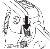
**NOTE!** The start/stop switch automatically returns to run position. In order to prevent unintentional starting, the spark plug cap must be removed from the spark plug when assembling, checking and/or performing maintenance.
