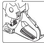
As the chain brake is still activated the engine must return to idling speed as soon as possible by disengaging the throttle latch in order to avoid unnecessary wear on the clutch assembly.
