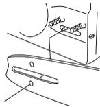
Tension the chain by turning the chain tensioning screw clockwise using the combination spanner. See instructions under the heading Tensioning the chain.
