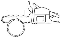
There are methods for felling trees with a diameter larger than the bar length. However these methods involve a much greater risk that the kickback zone of the bar will come into contact with the tree.
