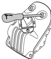
Some mufflers are equipped with a special spark arrestor screen. If your machine has this type of muffler, you should clean the screen at least once a week. This is best done with a wire brush. A blocked screen will cause the engine to overheat and may lead to serious damage.
