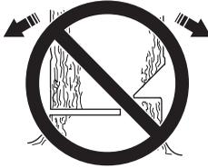
When the felling cut and directional cut are complete the tree should start to fall by itself or with the aid of a felling wedge or breaking bar.
