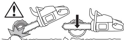
If it is possible (can you turn the log?) stop cutting about 2/3 of the way through the log.
