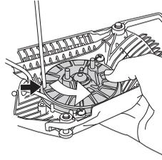
Remove the clip in the centre of the pulley. Remove the spacer and the pulley. Insert and fasten a new starter cord onto the pulley. Wind approx. 3 turns of the starter cord onto the pulley. Connect the pulley to the recoil spring so that the spring engages in the pulley. Fit the spacer and secure the pulley with the clip. Insert the starter cord through the hole in the starter housing and the starter handle. Make a secure knot in the end of the starter cord.
