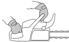
Apply full throttle and activate the chain brake by tilting your left wrist forward onto the front hand guard. Do not let go of the front handle. **The chain should stop immediately.**
