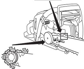
Make sure that the edges of the cutting links are facing forward on the top edge of the bar.
