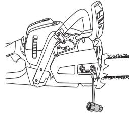
The chain is correctly tensioned when it does not sag from the underside of the bar, but can still be turned easily by hand. Hold up the bar tip and tighten the bar nuts with the combination spanner.
