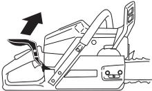
Push the trigger up and forwards to check that it moves freely and is securely hinged to the clutch cover.
