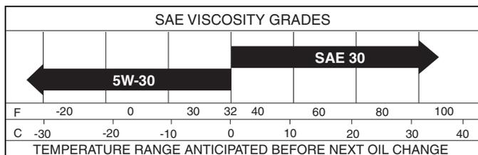
**NOTE:** Although multi-viscosity oils (5W30, 10W30 etc.) improve starting in cold weather, they will result in increased oil consumption when used above 32°F/0°C. Check your engine oil level more frequently to avoid possible engine damage from running low on oil.
