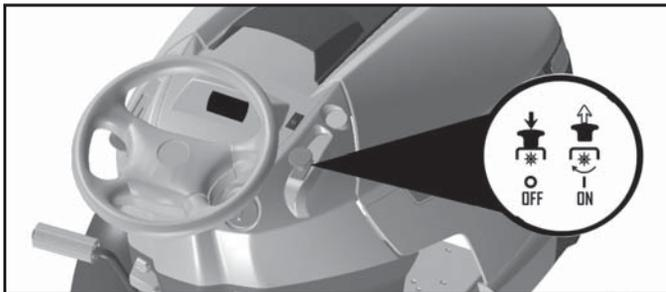
(☒) ATTACHMENT CLUTCH SWITCH "DISENGAGED"
