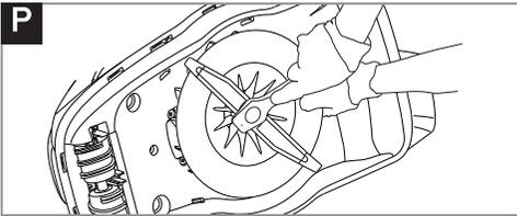
Always handle the blade with care - sharp edges could cause injury. USE GLOVES. Never use more than 3 Cutting Height Spacers. Spacers must only be fitted between the blade and the fan and NEVER between the blade and the bolt.
