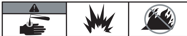
Battery acid is corrosive, explosive and flammable
