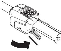
Press the power trigger and make sure it returns to its original position when you release it.
