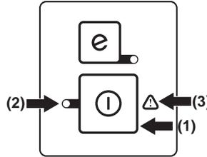
Flashing warning symbol (3) and green LED (2) is lit could indicate that:
