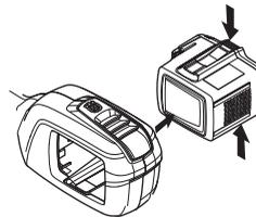
**IMPORTANT!** Always remove the battery to prevent the machine being started by accident.
