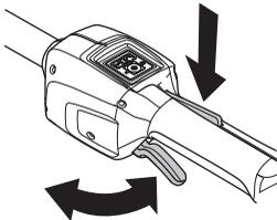
See instructions under the Start heading. Start the machine and apply full power. Release the power trigger and check that the cutting attachment stops and remain at a standstill.
