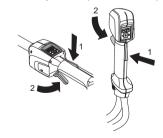
Make sure the power trigger is locked when the power trigger lock is in its original position.
