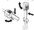
See instructions under the Start heading. Start the machine and apply full power. Release the power trigger and check that the cutting attachment stops and remain at a standstill.
