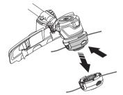
· Pull out the line chute assembly.
