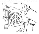
**CAUTION!** Never use a machine with a defective muffler. Check regularly that the muffler is complete and secured correctly. Tightening torque 7 - 10 Nm
