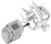
Press on the lower part of the battery and push it in as far as it will go into the battery compartment. Make sure the latches snap in place properly.
