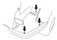
2 Loosen the locking nuts (1).
