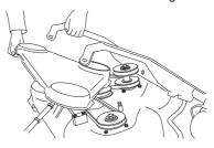
8 Loosen the spring that tensions the V-belt and pry off the belt.
