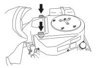
2 Loosen the hose clip that holds the filter cartridge.
