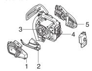
Clean the cooling system with a brush once a week, more often in demanding conditions. A dirty or blocked cooling system results in the machine overheating which causes damage to the piston and cylinder.
