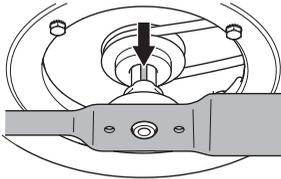
Fit the spring washer and tighten the bolt and washer correctly. The bolt must be tightened with a torque of 45-60 Nm.
