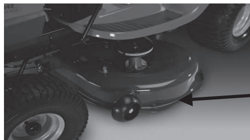
Stamped Deck Shell below, NOT reinforced
