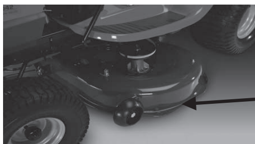
Stamped Deck Shell below, NOT reinforced
