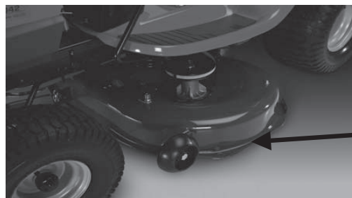
Stamped Deck Shell below, NOT reinforced
