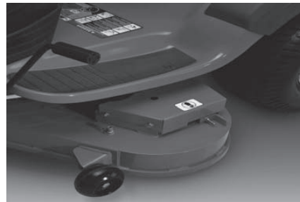
Fabricated Deck Shell Example Below
