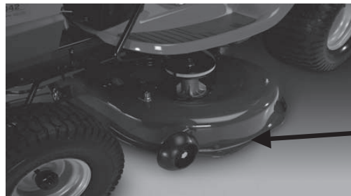
Stamped Deck Shell below, NOT reinforced
