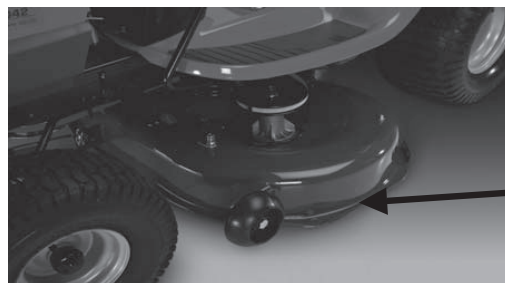
Stamped Deck Shell below, NOT reinforced
