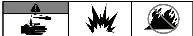
Battery acid is corrosive, explosive and flammable
