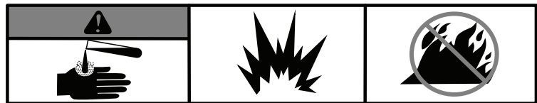
Battery acid is corrosive, explosive and flammable
