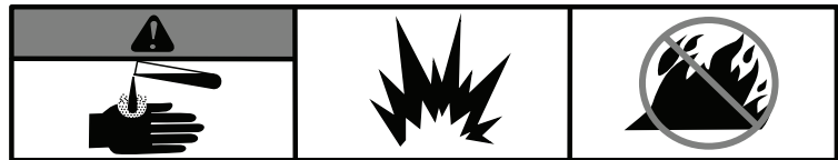
Battery acid is corrosive, explosive and flammable
