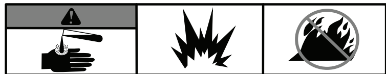
Battery acid is corrosive, explosive and flammable
