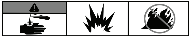
Battery acid is corrosive, explosive and flammable
