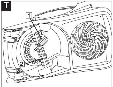
**Switch off, wait until the blade has stopped rotating and disconnect from the mains electricity supply BEFORE attempting to remove or refit the blade.**
