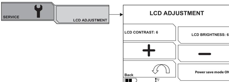
Use the arrows up and down to adjust the display's contrast and brightness.
