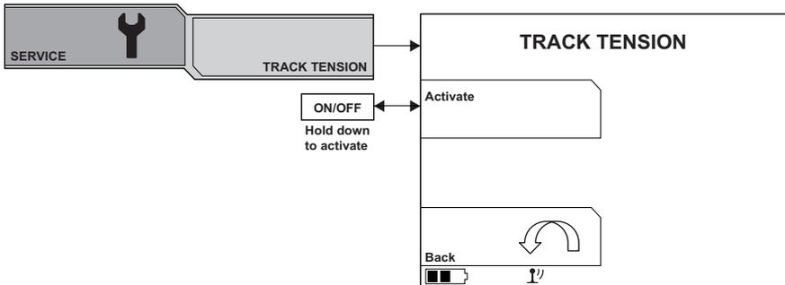
Hold the selection key down to activate the track tension.
